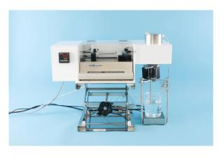
On the picture above you see the contained vessel of VAR A with the heating chamber.
